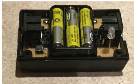
Open the case by removing the four screws. Hold down the small push switch and turn the unit on. The LED will briefly flash red/green then show steady green. Now send the appropriate system exclusive file to the unit from a suitable PC/Mac program\*. As data is received the LED will flash green and finally the unit will re-boot. Close the box, replace the screws and enjoy!
